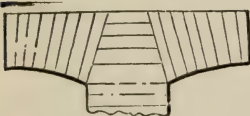
Fig. 79—Represents a mode of arranging the voussoirs and horizontal courses in flat segment arches.
